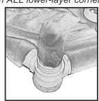
Step 2b: Ensure screw enters the fabric opening on ALL lower-layer corners
